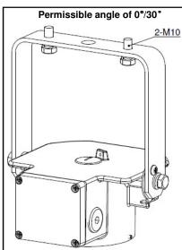
Fig. 1 Luminiare adjustment for bracket mounting
